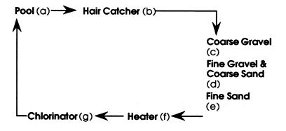
Figure 1. Swimming Pool Filter System
